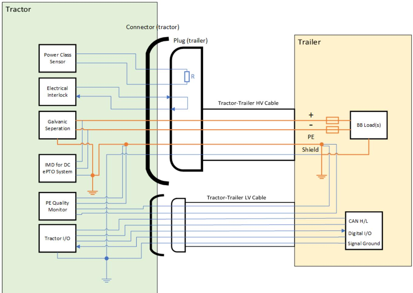
Figure 4 HV and LV connectors
