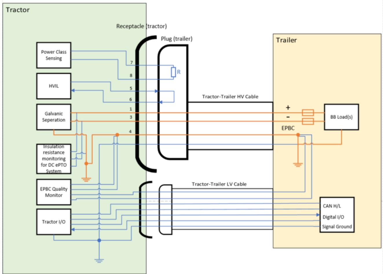
Figure 2 HV and LV connectors
