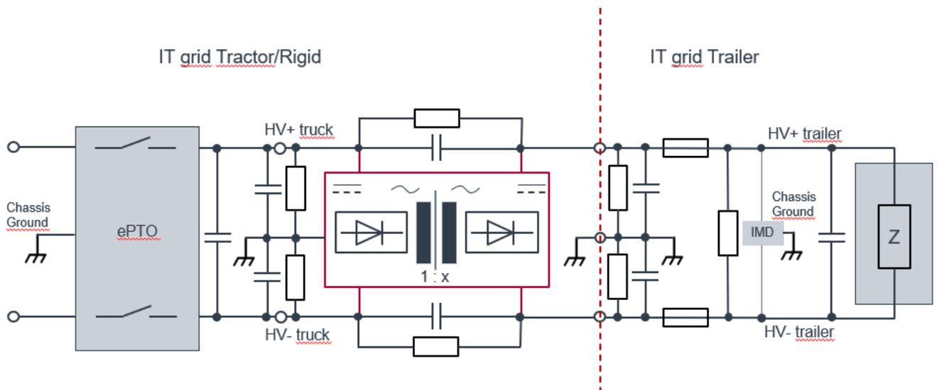
Figure 1 Wiring diagram for HV galvanic separation of truck and trailer
