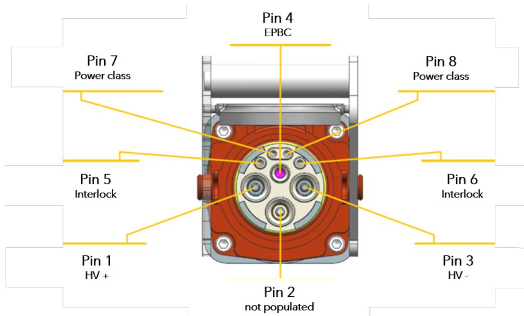
Figure 1: Example based on the ISO 23316-1
