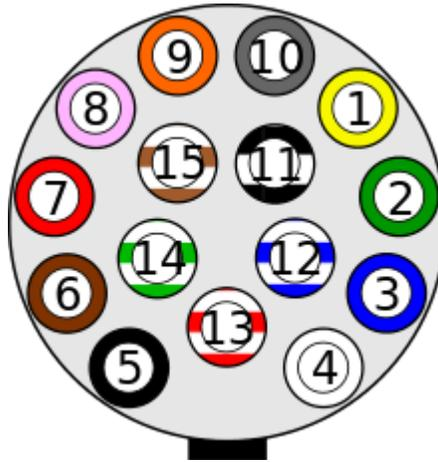
Figure 4: LV Connector acc. ISO 12098
